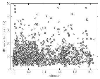
**Figure 7.** Air mass versus RV uncertainty per spectrum. Typically, targets are observed when they are close to the meridian passage, but this is not always possible owing to scheduling constraints. It is clear that RV uncertainty is not systematically affected by the air mass at which the K dwarfs have been observed.
