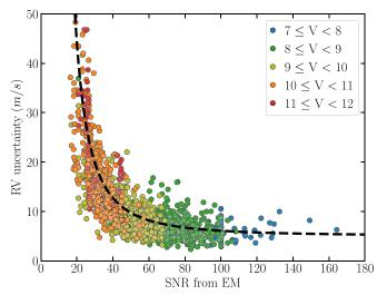
**Figure 6.** S/N calculated from CHIRON's exposure meter (EM) vs. RV uncertainty for individual spectra, color-coded by stellar V magnitude. Each of the 1784 data points represents a single spectrum. The dashed line is described by Equation (1) and is derived using observations with exposure times of 900 s. The slight overabundance of points at S/N = 100 is the result of observations that were stopped before 900 s, when the S/N reached 100.
