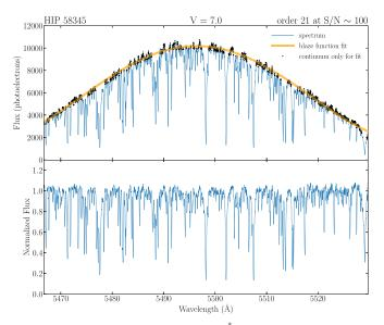
**Figure 2.** Spectrum of order 21 ( $\sim$ 5460–5530 Å) of HIP 58345 taken in slicer mode ( $R \sim 80,000$ ) at S/N  $\sim$ 100. Top: spectrum before the removal of the blaze function, where the black circles are the data points from the original spectrum (blue line) used to fit the blaze function (yellow line). Bottom: normalized spectrum after the removal of the blaze function.
