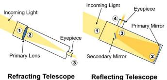
consists of a primary mirror at the base of the tube which reflects the light to a secondary mirror which reflects the light out to the eyepiece.
