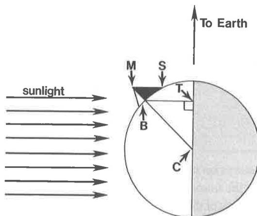
**Fig. 1:** Geometry used to determine the height of a lunar mountain.
