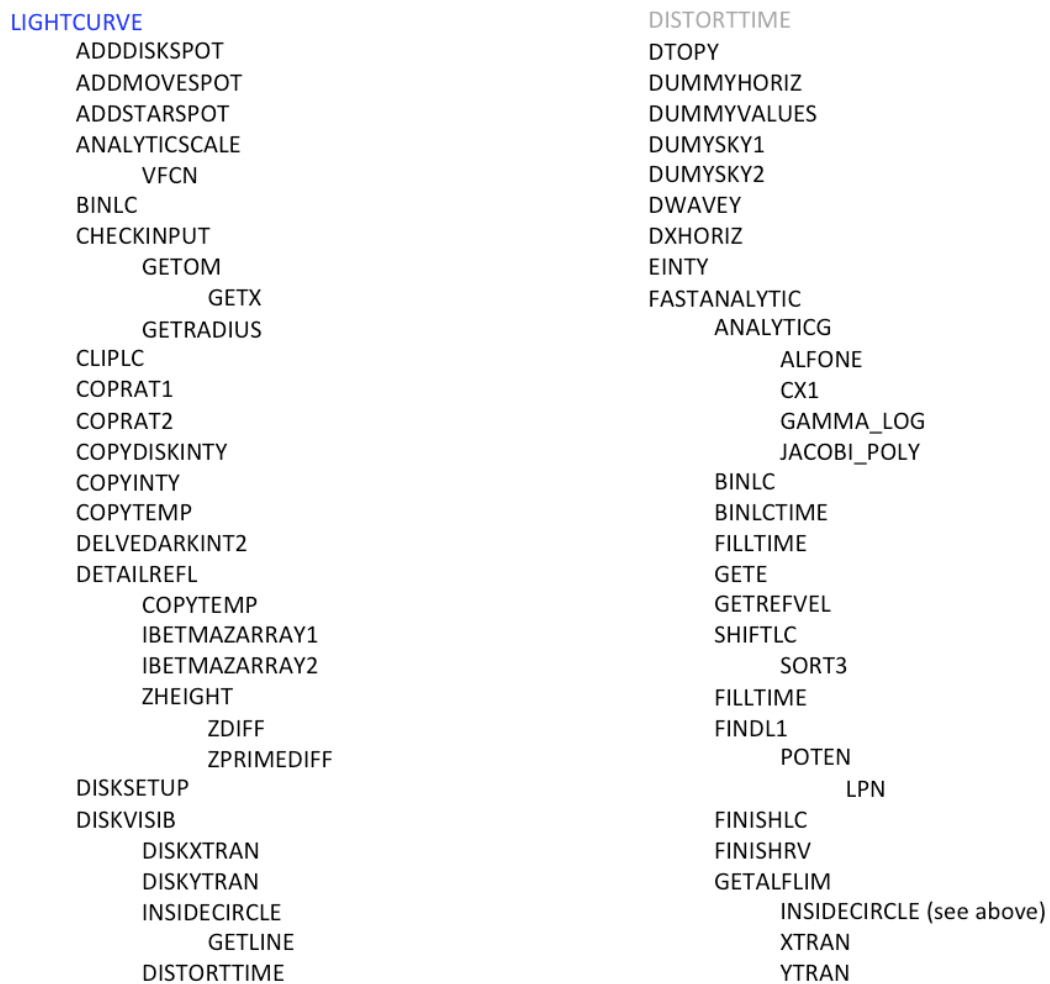
Figure C.1 Call tree of the subroutine lightcurve in ELC.
