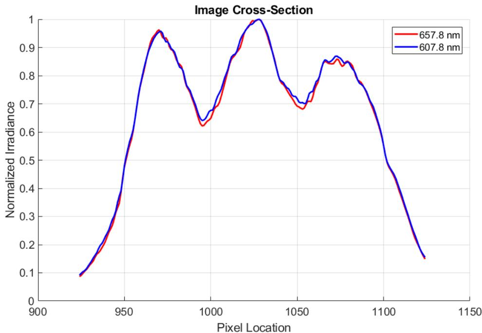
Figure 4: Cross section of irradiance in the image plane of the optical system. The figure cuts through a horizontal section of the output so that all three bars can be clearly seen. This is done for two separate wavelengths (50nm apart) to show that the simulation is behaving as expected. It can be clearly seen that in between the bars there is more irradiance in the bluer wavelength.
