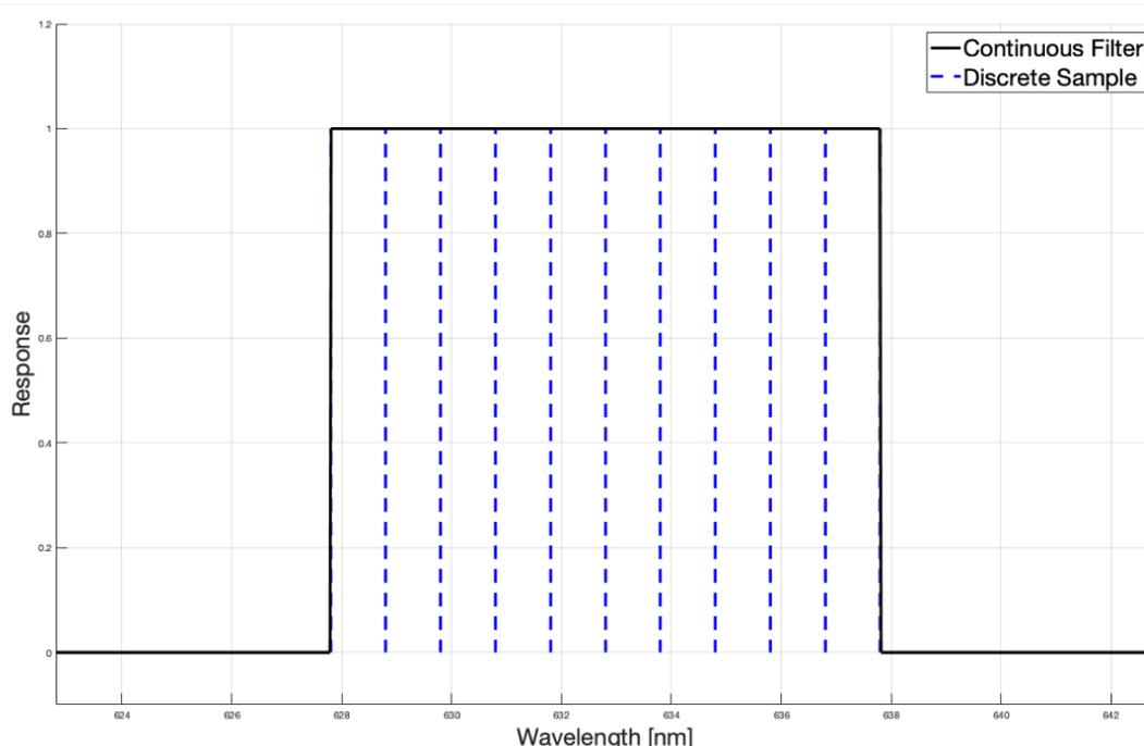
Figure 1: Example of the Spectral Slicing method on a square response filter centered at a wavelength of 632.8nm. This example includes a total width of 10nm with 1nm sampling.
