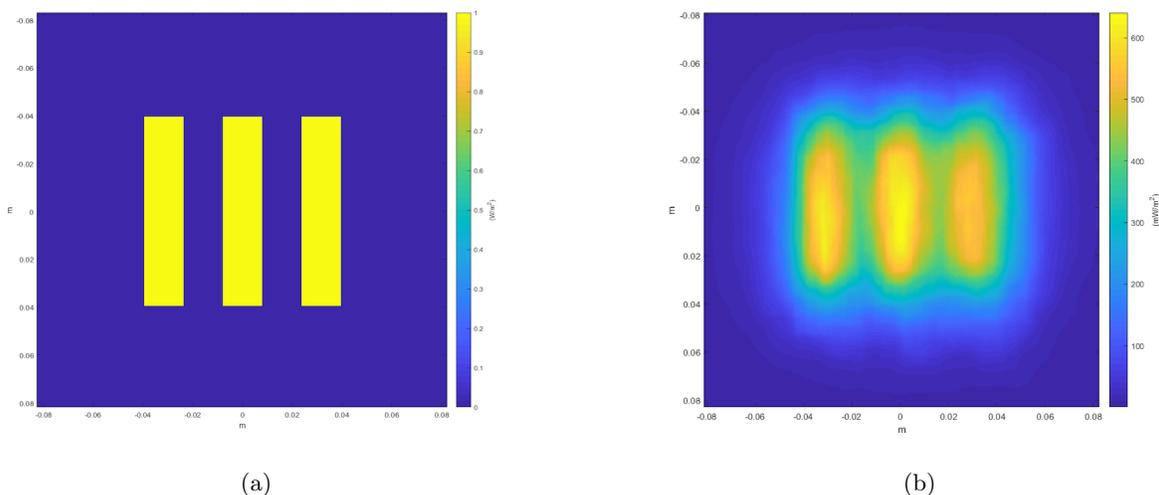
Figure 2: The effects of anisoplanatism. (a) shows the three bar target amplitude in the object plane (no propagation). (b) shows the three bar target amplitude in the image plane after propagation through distributed-volume atmospheric turbulence. The results presented here are for the central wavelength given in Table 1.
